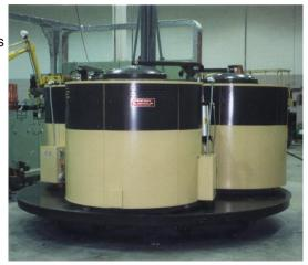
THERMTRONIX® builds added value into every furnace with features like: Pneumatic furnace lid with operator hand/foot valve; ground fault system and integral over-current protection circuit breaker for total high voltage isolation; three direct reading ammeters. Powerguard™ control system assures maximum performance and extended heating element life. Immersion thermocouple and solid state controller automatically adjusts metal temperatures. Metal leak detector system indicates metal leakage.
