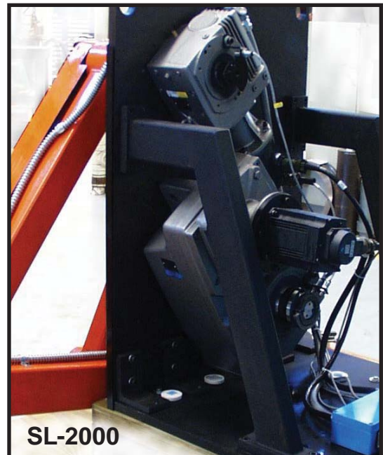
Direct drive systems with servo motor and encoder mounted directly to the gear box.
