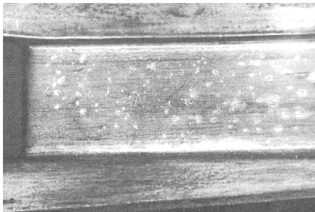
Fig. 9-10. Heat marks usually occur in depressed areas on the casting. Depressed areas are formed into the casting by raised areas in the die, and such parts of the die tend to mil hot.
