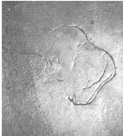
Fig: 9-7 Severe chill is usually the result of a cold die. Die cooling water flow in the area should be reduced until the chill disappears.
