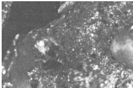
Fig. 9-27. Flux inclusions cause problems with coatings and adhesives identified by a gray crystalline appearance.
