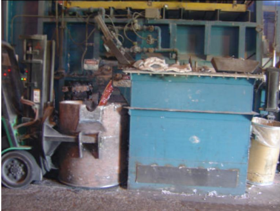
Figure 16 Tapping out molten metal by pressurizing a side chamber with air
