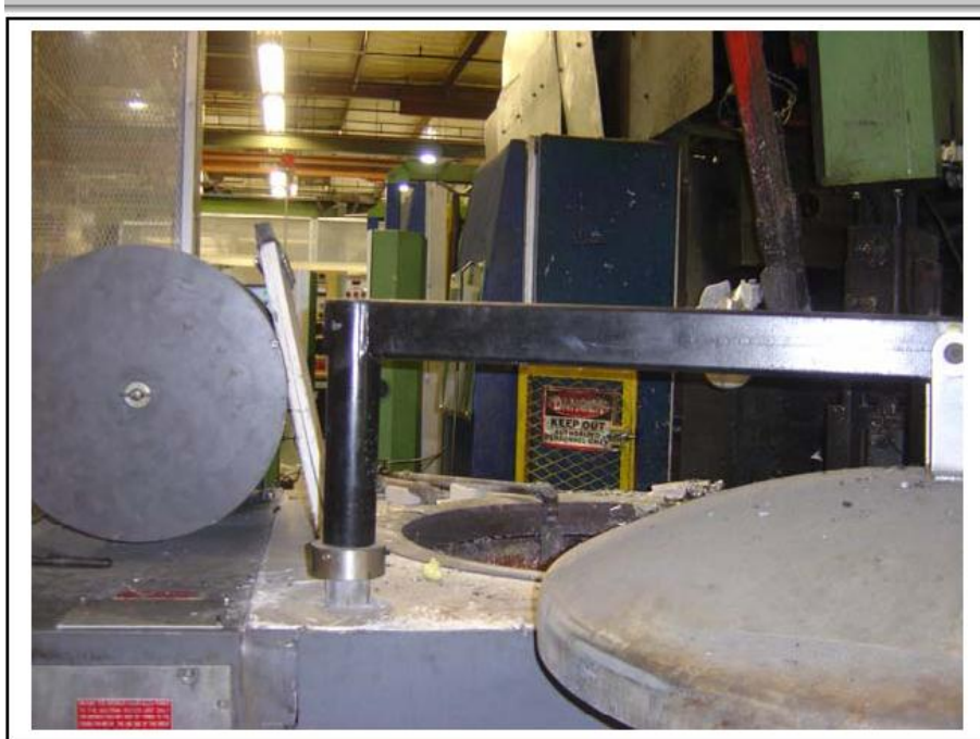
Figure 23 Inductotherm Acutrak DEH induction aluminum melting furnace
