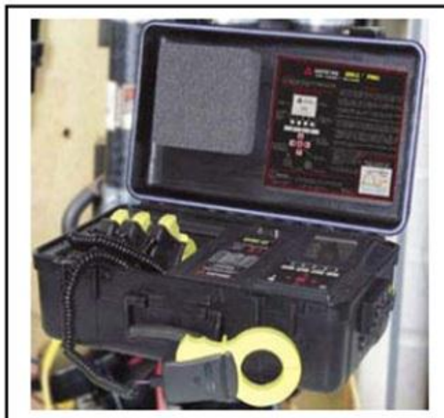
Figure 24 Ampco DM-II Pro power analyzer
