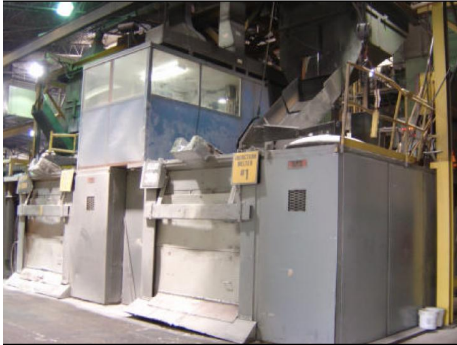
Figure 17 Coreless induction furnaces at Mercury Marine
