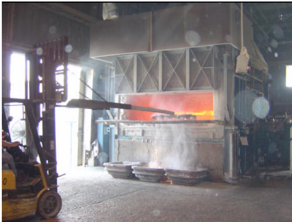
Figure 15 Charging ingots/skimming through the front door of a gas reverberatory furnace.
