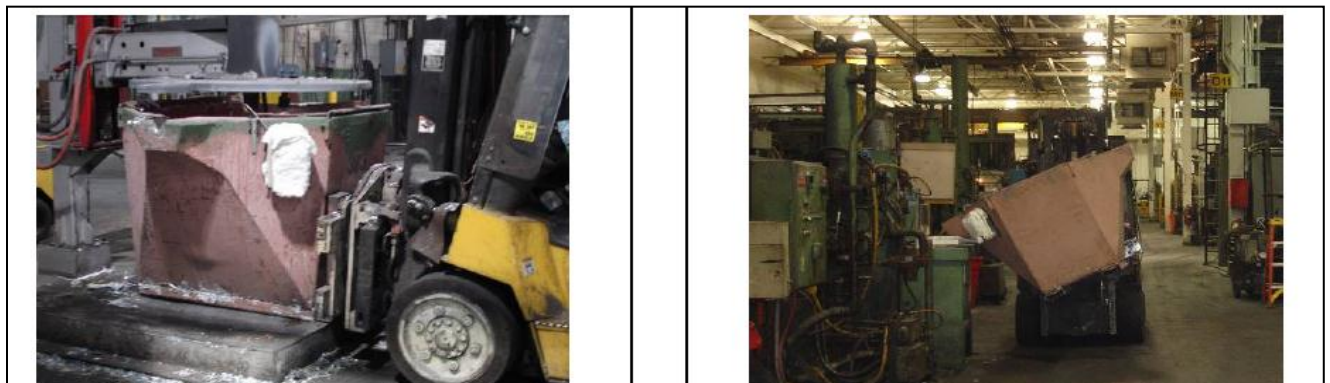
Figure 7 Degassing (L) and Tapping Metal (R)
