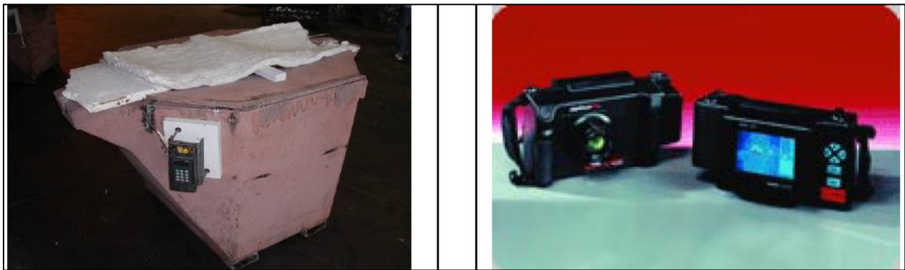
Figure 8 Covered Ladle (L) and Infrared Camera (R)
