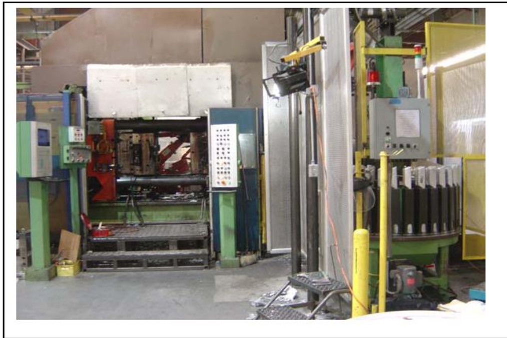
Figure 22 Die casting cell with ingot loader
