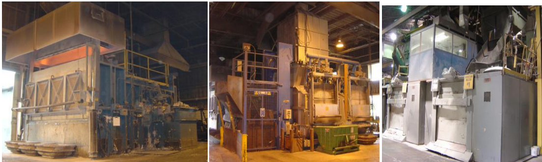
Figure 1 Three of the large Benchmarked Melting Furnaces: left to right reverberatory, stack and induction.
