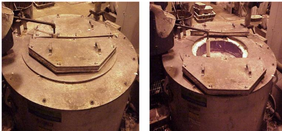
Figure 3 Covered 75kW furnace (L) and Uncovered 75kW furnace (R)
