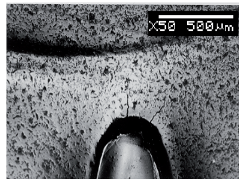
Fig. 6. Working surface of the testing die-casting die. Surface pits and cracks at identification mark. OM
