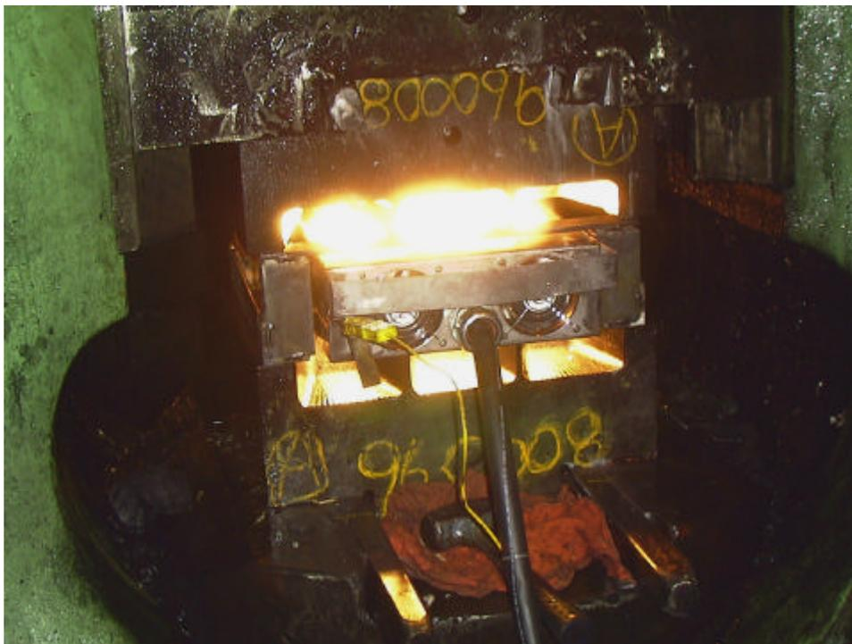
Figure 10. Oak Ridge National Laboratory insert heater preheats hammer forge dies at KomTek.
